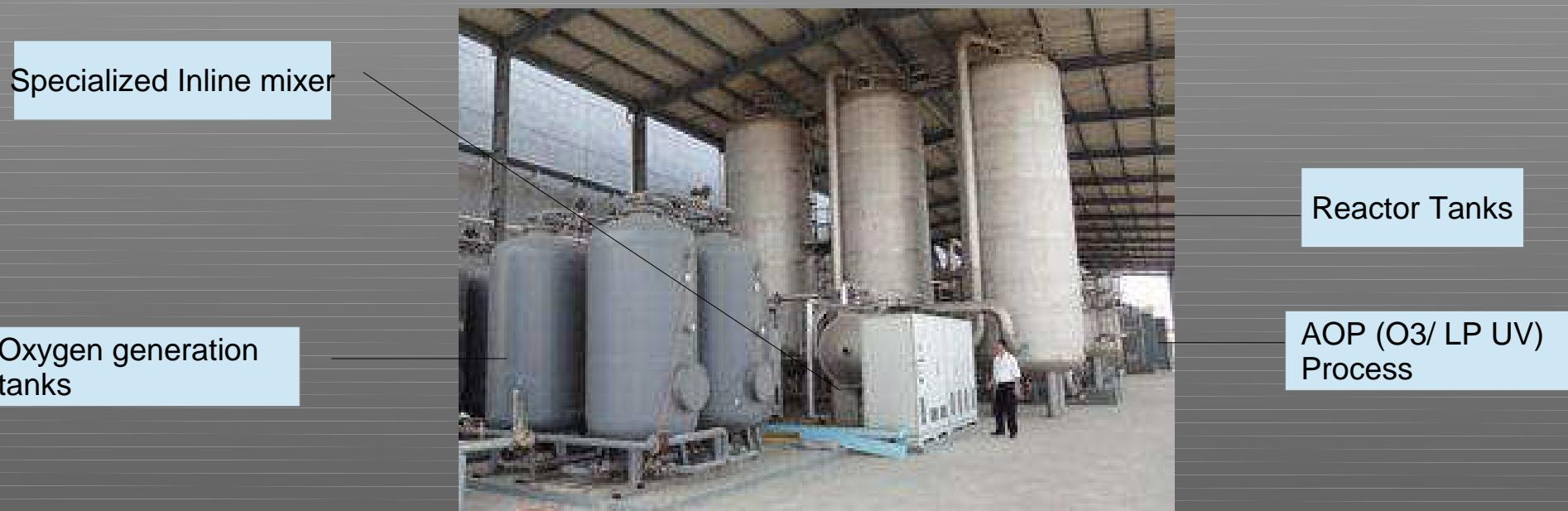
The creation of reactive particles (OH) with the highest oxidant value are generated to specifically target the compounds in the stream. In this secondary or tertiary treatment process.
